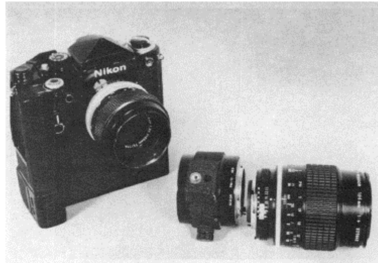
Fig 1.—At left is Nikon camera fitted with motor drive and 55-mm macro lens. This unit is used for 23 of 24 photographs. At right are Micronikkor (Nikon) 105-mm lens and Pn11 extension tube that are used for photographing the 1:1 image.
